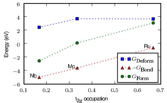
FIG. 2. (Color online) The formation energy, the metal bulk deformation energy, and the bonding energy in the expanded metal lattice as functions of the filling of the metal  $t_{2g}$  band for some representative rutile  $4d$  metal dioxides (Nb, Mo, and Ru). The variation in formation energy is clearly dominated by the oxygen binding energy.
