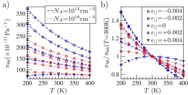
FIG. 4. (Color online) Piezocoefficient  $\pi_{66}$  as a function of temperature for different magnitudes of the grown-in biaxial strain. Results are shown for two different dopant densities. Results in (b) are shown relative to the value of  $\pi_{66}$  at  $T=300$  K. Note that the legend is spread across both figures.
