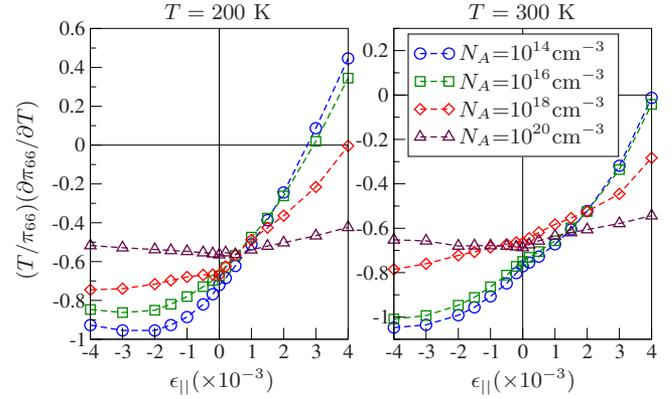
FIG. 5. (Color online) Temperature dependence of  $\pi_{66}$  as a function of the magnitude of the grown-in biaxial strain for four different dopant densities. Results are shown for temperatures of  $T=200$  K and  $T=300$  K, respectively. Note the different scales on the ordinates of the two figures.
