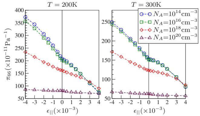
FIG. 2. (Color online) Piezocoefficient  $\pi_{66}$  as a function of the magnitude of the grown-in biaxial strain for four different dopant densities. Results are shown for temperatures of  $T=200$  K and  $T=300$  K, respectively. Note the different scales on the ordinates of the two figures.
