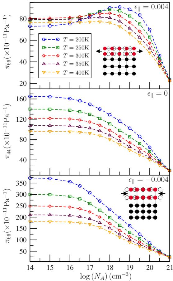
FIG. 1. (Color online) Shear piezocoefficient  $\pi_{66}$  as a function of temperature and dopant density. Results are shown for silicon and for strained silicon with a grown-in biaxial strain of  $\epsilon_{||}=0.004$  (tensile) and  $\epsilon_{||}=-0.004$  (compressive), respectively. The panel in the middle shows the shear piezocoefficient for unstrained silicon where  $\pi_{66}=\pi_{44}$ . The insets illustrate the fabrication of strained silicon layers.
