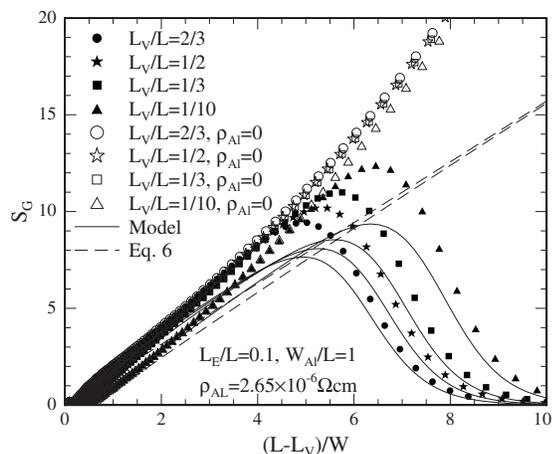
FIG. 3. Geometrical amplification  $S_G$  as a function of  $(L-L_V)/W$  calculated using the COMSOL FEM model. Data from calculations using  $L_E/L=0.1$  and  $L_V/L \in [1/10, 1/2, 1/2, 2/3]$  (symbols  $[\blacktriangle, \blacksquare, \star, \bullet]$ ) are shown along with the simple model [Eq. (6)] (dashed lines), as well as a model using Eqs. (8) and (10) corrected for finite Al resistivity (full lines). The corresponding open symbols signify FEM data assuming zero metal resistivity.
