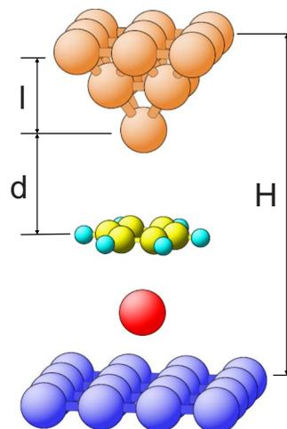
FIG. 1. (Color online) Setup for the calculations.  $H$  is the distance between the magnetic STM tip and the substrate.  $l$  is the length of the tip, while  $d$  is the distance between the benzene molecule and the tip apex.
