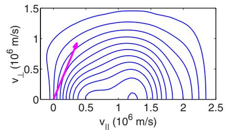
FIG. 15. (Color online) Fokker-Planck simulation of beam ions for TEXTOR shot No. 89509 at the NBI flat top at  $t=2.1$  s. The contour levels are equispaced. The cylindrical coordinates  $v_{\parallel}$  and  $v_{\perp}$  represent the direction antiparallel and perpendicular to the static vacuum magnetic field. The direction of the projection measured by CTS,  $67^\circ$  to  $v_{\parallel}$ , is indicated by the arrow.
