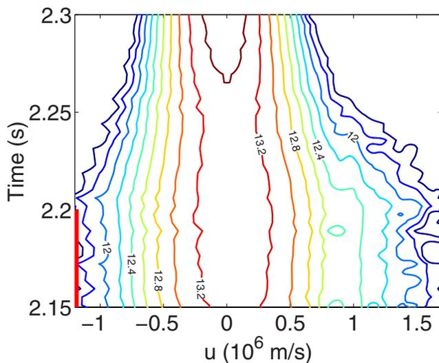
FIG. 19. (Color online) Time evolution of the measured 1D velocity distribution ( $\log_{10} f^{1D}$ ). The fast ions seen at  $u=1-1.5 \times 10^6$  m/s decay once the ion heating is turned off at  $t=2.2$  s.
