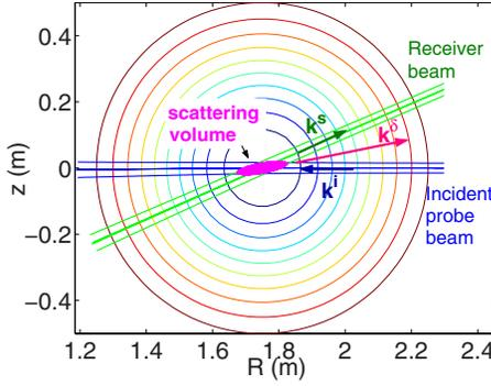
FIG. 1. (Color online) CTS scattering geometry in the TEXTOR tokamak. The probe enters the plasma in the horizontal midplane and the first receiver mirror is located  $\sim 20$  cm above. The resolved fluctuation wave vector  $\mathbf{k}^\delta = \mathbf{k}^s - \mathbf{k}^i$  is generally pointing towards the launch and receiver mirrors for the back scattering geometry used on TEXTOR.
