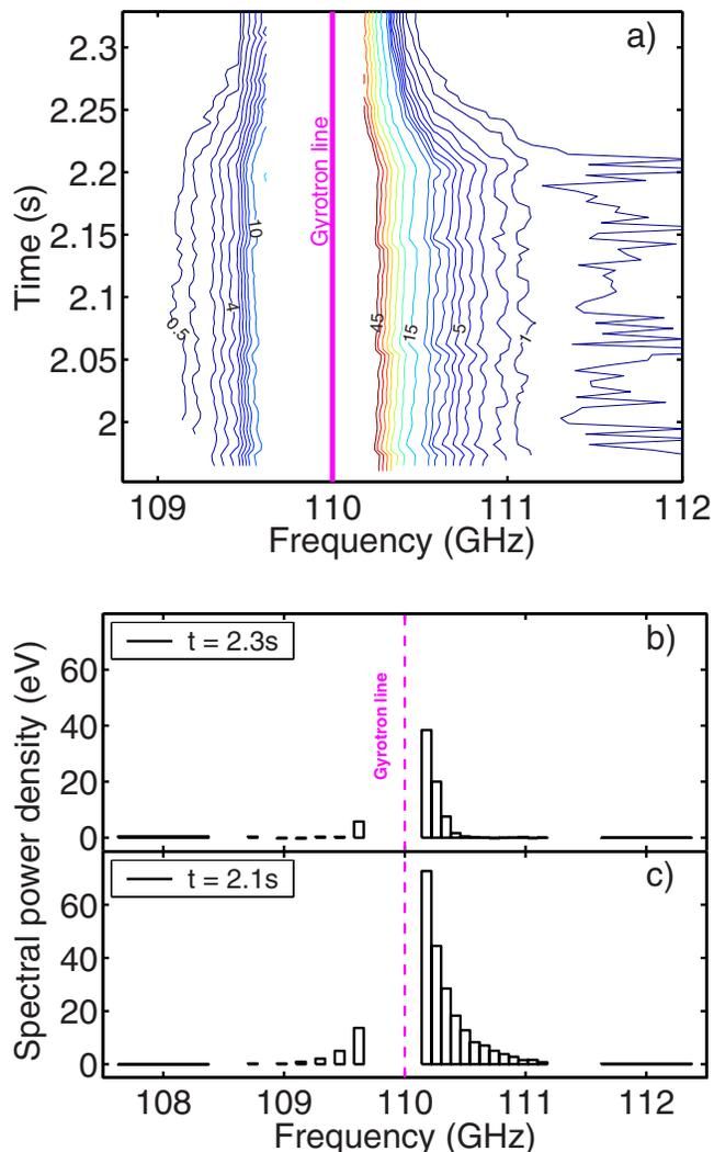
FIG. 5. (Color online) Contour plot of CTS spectral power density (a). The width of the CTS spectrum is seen to decrease after the ion heating is turned off at  $t=2.2$  s. CTS spectrum at  $t=2.3$  s (after heating turn off) is shown in the upper plot (b) while that at  $t=2.1$  s (during heating flattop) is shown in the lower plot (c).
