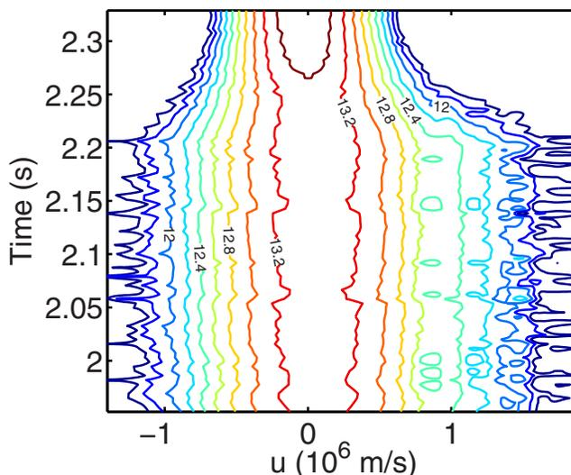
FIG. 11. (Color online)  $\text{Log}_{10}$  contour plot of obtained velocity distribution. The scattering geometry is described in Sec. III with a radial position of  $R=1.67$  m and a resolved direction of  $113^\circ$  to the magnetic field.
