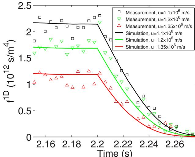
FIG. 18. (Color online) Direct comparison of measurement and simulation at superthermal velocities. As shown in Fig. 9(b) the ion population densities at  $u=1.1, 1.2$  and  $1.35 \times 10^6$  m/s extend the bulk distribution. Good agreement during the slowing-down phase is found.
