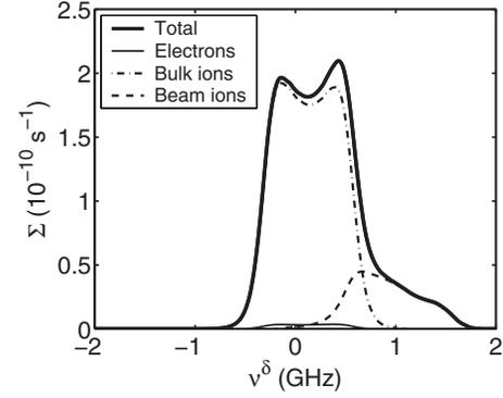
FIG. 2. Theoretical scattering function  $\Sigma$  for a neutral-beam-heated TEXTOR plasma. The resolved velocity component makes an angle of  $160^\circ$  to the static magnetic field. The plasma parameters are  $n_e = 3 \times 10^{19} \text{ m}^{-3}$ ,  $T_e = T_i = 2 \text{ keV}$ ,  $n_D = 2.5 \times 10^{19} \text{ m}^{-3}$ ,  $n_H = 2 \times 10^{18} \text{ m}^{-3}$ , and  $n_{\text{beam ion}} = 3 \times 10^{18} \text{ m}^{-3}$ .
