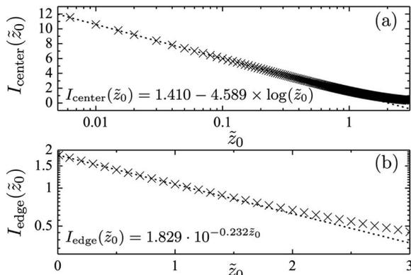
FIG. 6. Values of (a)  $I_{\text{center}}(\tilde{z}_0)$  and (b)  $I_{\text{edge}}(\tilde{z}_0)$  calculated as a function of  $\tilde{z}_0$  as described in the text. The dotted lines and the written equations are analytical approximations valid for low values of  $\tilde{z}_0$ .
