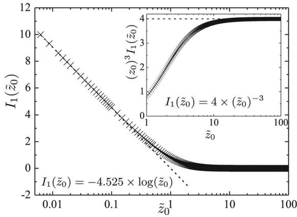
FIG. 5. Values of  $I_1(\tilde{z}_0) = -(H_{by}(\tilde{z}_0)) / (\chi H_{ext} \tilde{R} / 3\alpha)$  calculated for a square sensor ( $\ell=1$ ) as a function of  $\tilde{z}_0$ . The inset shows  $(\tilde{z}_0)^3 I_1(\tilde{z}_0)$  for large values of  $\tilde{z}_0$ . The dashed lines are the indicated simple analytical approximations.
