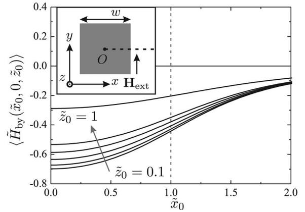
FIG. 2. Normalized average magnetic field in the  $y$ -direction from a single bead at the position  $(\tilde{x}_0, 0, \tilde{z}_0)$  of a square sensor ( $\ell=1$ ) as a function of  $\tilde{x}_0$  for  $\tilde{z}_0=0.1, 0.2, 0.3, 0.4, 0.5, 1$  (increasing values indicated by arrow). The sensor edge is at  $\tilde{x}_0=1$ . The inset shows the sensor geometry; the investigated values of  $\tilde{x}_0$  are indicated by the dashed line.
