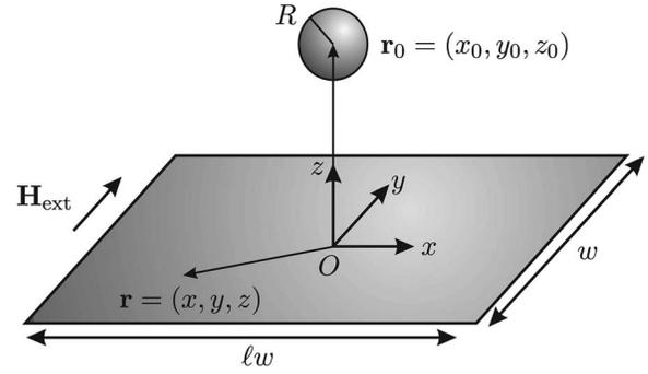
FIG. 1. Sketch of the system of interest: The external magnetic field is chosen to be fixed in the  $y$ -direction. The sensor is in the  $xy$  plane and has side lengths  $\ell w$  and  $w$  in the  $x$ - and  $y$ -directions, respectively. The origin ( $O$ ) of the coordinate system is in the center of the sensor.
