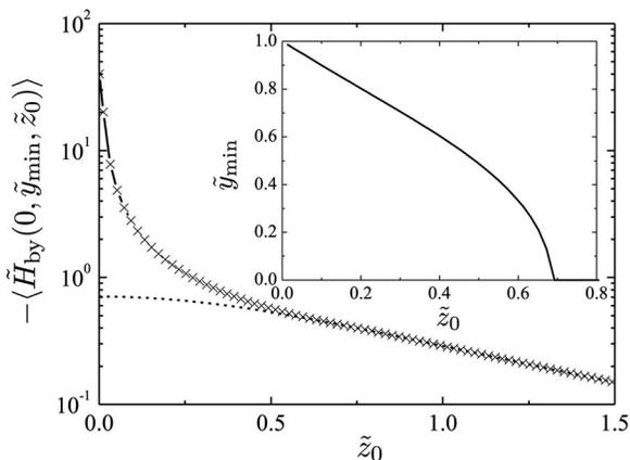
FIG. 4. Minimum average magnetic field as a function of  $\tilde{z}_0$  for a square sensor. The dashed line corresponds to the average magnetic field from a bead position above the center of the sensor [Eq. (11)]. The inset shows the position of the minimum as a function of  $\tilde{z}_0$ .
