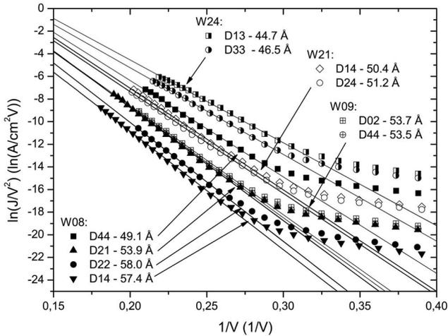
FIG. 5. The  $I$ - $V$  characteristics from Fig. 4 shown in a Fowler plot. The data yield straight lines in the Fowler-Nordheim regime above 3.4 V, corresponding to  $\sim 0.29$  on the inverse voltage axis. The slope of the Fowler-Nordheim fit should be proportional to the thickness, as seen from Eq. (6).
