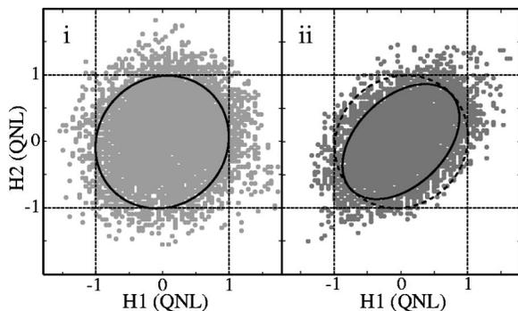
FIG. 3. Correlation between the photocurrents of  $H1$  and  $H2$  at 4.5 MHz for (i) vacuum noise and (ii) amplitude squeezing incident on the beam splitter. The quantum noise is shown for reference. The ellipses are the square root of the conditional variance, normalized to the QNL. The data is not to scale with the radii of the curves.
