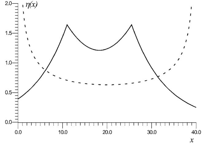
FIG. 1. The distribution of overlap component of bias current  $\eta(x)$ . Short-dashed line:  $\eta(x) = \frac{\eta_0 L}{\pi \sqrt{x(L-x)}}$ ; solid curve:  $x_0 = 11$ ,  $x_1 = 25.5$ ,  $p = 0.13$ , and  $a = 0.005$ .
