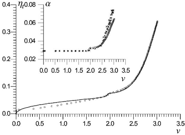
FIG. 4. Current-voltage characteristics of the FFO. Thin line—experimental measurements. Numerical simulations including the self-pumping effect—circles. Inset: the damping factor  $\alpha(x)$  at the middle of the junction (crosses) and spatially averaged over  $x$  (circles).
