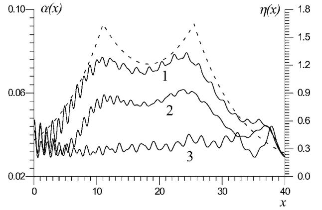
FIG. 5. Spatial dependence of the shunt damping  $\alpha(x)$  for three currents  $\eta_i$ ;  $\Gamma = 3.7$ : curve 1,  $\eta_i = 0.3$ ; curve 2,  $\eta_i = 0.2$ ; and curve 3,  $\eta_i = 0.1$ . The dashed line represents the distribution of  $\eta(x)$ .
