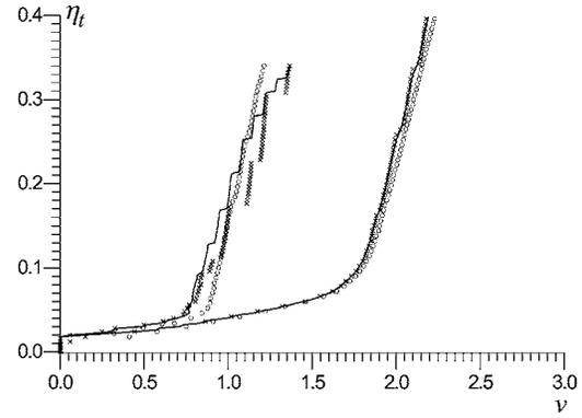
FIG. 3. Calculated current-voltage characteristics of the FFO. Numerical simulations for different values of the load; crosses, unloaded symmetrical case; thin lines, asymmetric load  $r_L=2$ ,  $r_R=100$ ; and circles, perfect matching  $r_L=r_R=1$ ; all other parameters are the same as used for the IVCs in Fig. 2.
