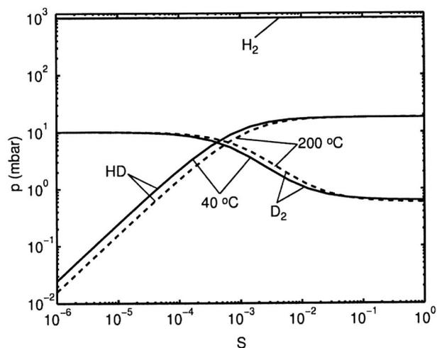
FIG. 2. The calculated partial pressures of  $H_2$ , HD, and  $D_2$  at the capillary leak as a function of the sticking probability  $S$  at 40 (solid curves) and 200 °C (dashed curves). The gas mixture consists of 1%  $D_2$  in  $H_2$  at 1 bar total pressure and the flow rate is 100 (ml/min) $_n$ . The capillary-surface distance  $Z_{cap}$  and the nozzle-surface distance  $Z_n$  are both 0.2 mm. The diameter of the metal spot is 1 mm.
