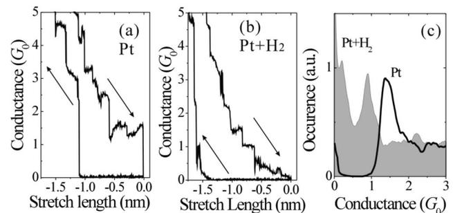
FIG. 1. Breaking and return traces for clean Pt (a), and for Pt in a H<sub>2</sub> atmosphere (b). Many of such curves are collected into conductance histograms as shown in (c) for clean Pt (black curve) and Pt in H<sub>2</sub> (filled graph).
