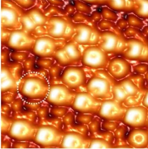
FIG. 1 (color online). Pseudo-three-dimensional representation of a constant-current STM image of Cu(100)-C<sub>60</sub> at 8 K. (Sample voltage  $V = 1.7$  V, tunneling current  $I = 1$  nA, scan size  $49 \text{ \AA} \times 49 \text{ \AA}$ ). A dashed circle indicates the C<sub>60</sub> orientation on which we performed the conductance measurements.
