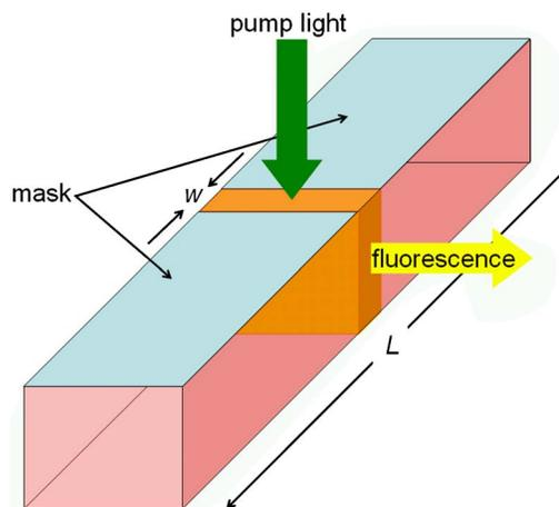
FIG. 1. Experimental setup. Closed channel containing a liquid solution of dye molecules. The dye molecules are optically pumped by a pulsed, frequency-doubled Nd:YAG laser through a slit of width  $w$  covering the sample.
