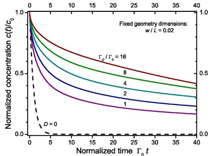
FIG. 2. Plot of dye molecule concentration vs time in a quasi one-dimensional microfluidic channel of length  $L$ , see Fig. 1. Bleaching by the optical pump occurs through a narrow slit of width  $w = 0.02L$  with a bleaching rate  $\Gamma_0$ . Diffusion changes the dynamics away from the pure exponential bleaching ( $D = 0$ ) and yields a much slower decay.
