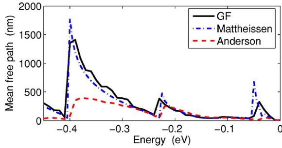
FIG. 8. (Color online) Mean free path vs energy for a concentration of vacancies corresponding to  $\langle d_H \rangle = 5.6$  nm. The solid black line corresponds to wires containing all possible vacancies. The dash-dotted blue line is obtained using Matthiessen's rule for single-scattering events and the dashed red curve corresponds to a wire with Anderson disorder ( $\Delta\varepsilon = 1.3$  eV).
