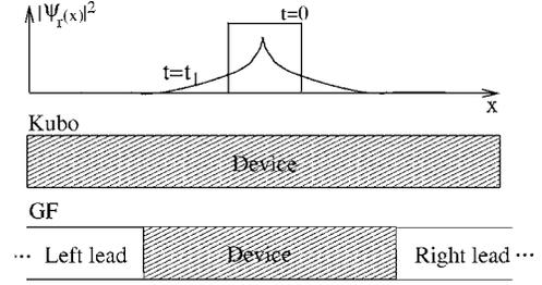
FIG. 1. Top: schematic time evolution of a random phase state  $|\psi_r(t)\rangle$  initially located in the central region of the wire. Middle: the geometry in the Kubo method consists only of a large device region. Bottom: in the GF approach a device region is connected to two semi-infinite leads.
