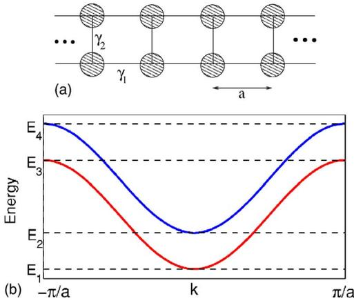
FIG. 10. (Color online) (a): model system. We consider only nearest-neighbor interaction with the tight-binding parameters  $\gamma_1$  and  $\gamma_2$  corresponding to hopping in the chain direction and in perpendicular direction, respectively. The on-site energy is  $\varepsilon_0$ . (b): band structure for the two bands separately. Notice the definition of the energies  $E_1$ – $E_4$ .
