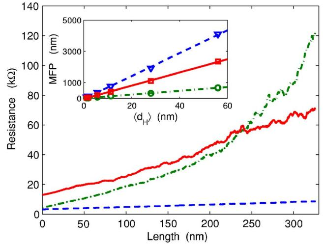
FIG. 9. (Color online) Length-dependent resistance at the energies  $E = -0.3$  eV (dashed blue line),  $E = -0.15$  eV (dash-dotted green line), and  $E = -0.03$  eV (solid red line). The average distance between vacancies is  $\langle d_H \rangle = 2.8$  nm. The inset shows the scaling of  $l_e$  vs average distance  $\langle d_H \rangle$  between vacancies at the same three energies as above.
