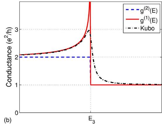
FIG. 11. (Color online). (a): the numerically calculated conductance (dash-dotted black line) is plotted together with the two analytical results  $g^{(1)}(E)$ , Eq. (A6) (dashed blue line) and  $g^{(2)}(E)$ , Eq. (A7) (solid red line). (b): zoom-in around  $E=E_3$ , showing that  $g^{(1)}(E)$  closely resembles the numerical result.
