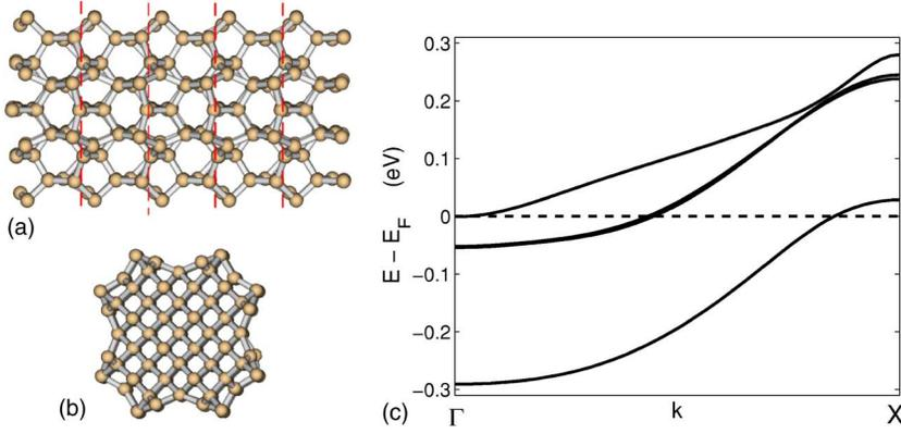
FIG. 4. (Color online) (a): Side view of the unpassivated SiNW containing five unit cells, separated by the red dashed lines. (b): End view of the unpassivated SiNW. (c): Band structure around the Fermi energy (dashed line). Four bands are crossing the Fermi energy, two being degenerate (with  $E - E_F = -0.05$  eV at the  $\Gamma$  point).
