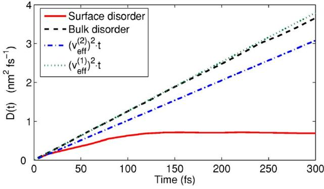
FIG. 5. (Color online) Time-dependent diffusion coefficient at  $E - E_F = 0.1$  eV. The bulk disorder has little effect and the transport is ballistic. The edge-disordered system shows diffusive behavior with a constant diffusion coefficient for  $t > 150$  fs.
