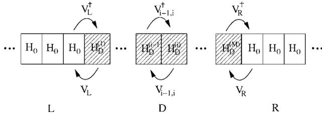
FIG. 2. The device region ( $D$ ) is divided into  $M$  subcells. The subcells are so large that they only couple to the nearest-neighbor cells. Also, the left ( $L$ ) and right ( $R$ ) leads consisting of equal unit cells, described by  $\mathbf{H}_0$ , couple only to the first and last cell of the device region, respectively.
