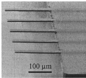
FIG. 1. Scanning electron microscopy image of an array of 200  $\mu\text{m}$  long cantilevers fabricated in the polymer SU-8. Cantilever width and thickness are 20 and 4.5  $\mu\text{m}$ , respectively.
