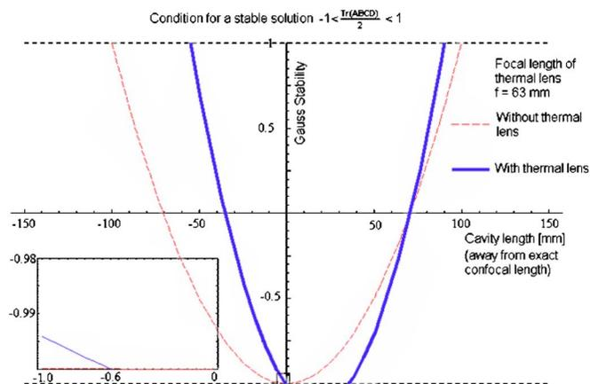
FIG. 2. (Color online) The Gauss stability as a function of cavity length change away from the exact confocal length. The thermal lens is  $f=63$  mm (pump power 1 W). The dashed curve is without thermal lens and the solid curve is with thermal lens. In the small box the deviation between the unpumped (without lens) and pumped (with lens) can be seen.
