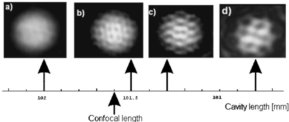
FIG. 9. The evolution of the complex signal far-field patterns as a function of the measured cavity length. (a)  $L=102.0$  mm. (b)  $L=101.5$  mm. (c)  $L=101.3$  mm. (d)  $L=100.8$  mm. All images are recorded with a gray filter. Observed confocal length 101.6 mm.
