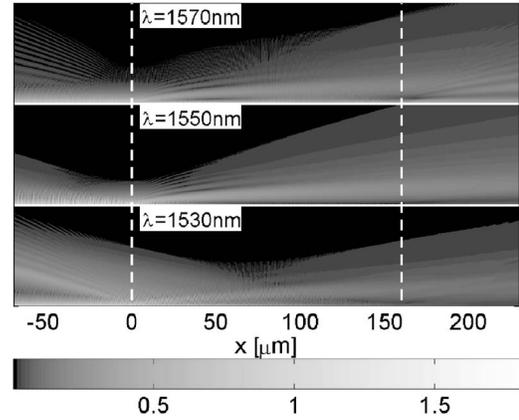
FIG. 5. Electric field magnitude versus height above and position along a LRSPG grating with 320 ridges of height 20 nm. The field magnitude is shown for three wavelengths,  $\lambda=1530$  nm ( $<$ bandgap),  $\lambda=1550$  nm (in bandgap), and  $\lambda=1570$  nm ( $>$ bandgap).
