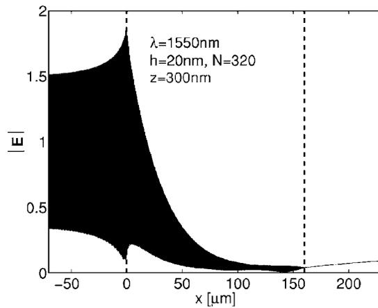
FIG. 6. Electric field magnitude versus position along a LRSPP grating with 320 ridges of height 20 nm. The fixed height  $y = 300$  nm above the gold film is considered. The wavelength is  $\lambda = 1550$  nm (in the bandgap).
