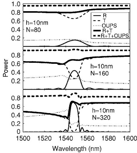
FIG. 2. Reflection ( $R$ ), transmission ( $T$ ), and out-of-plane scattering (OUPS) for LRSPG gratings with a 15 nm gold film and  $N=80, 160$ , and  $320$  gold ridges of height  $h=10$  nm, width  $W=230$  nm, and spacing  $\Lambda=500$  nm. The gold film and ridges are surrounded by a polymer with refractive index 1.543.
