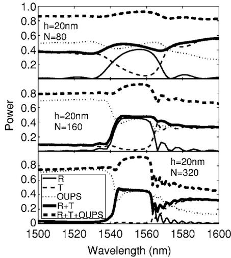
FIG. 4. Reflection ( $R$ ), transmission ( $T$ ), and out-of-plane scattering (OUPS) for LRSPG gratings with a 15 nm gold film and  $N=80, 160,$  and  $320$  gold ridges of height  $h=20$  nm, width  $W=230$  nm, and spacing  $\Lambda=500$  nm. The gold film and ridges are surrounded by a polymer with refractive index 1.543.
