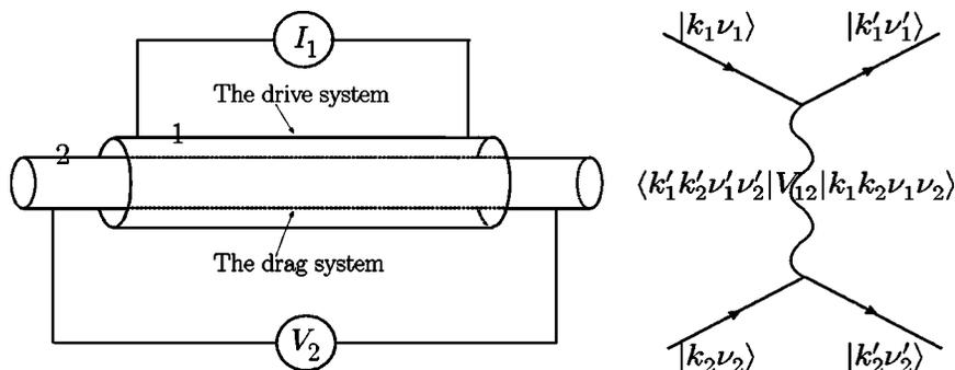
FIG. 1. (Left): The experimental setup to directly measure the Coulomb drag effect in a MWCNT. The intershell resistance is  $R_{21} = V_2/I_1$ . (Right): The basic mechanism in the intershell resistance in a drag configuration: the intershell  $e-e$  interaction and thereby momentum transfer to induce the voltage drop  $V_2$ .
