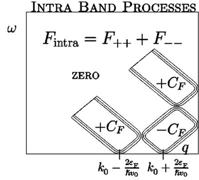
FIG. 6. Contour plot of the  $F_{\text{intra}}$  function.  $F_{\text{intra}}$  gives the phase space for intraband scattering in (real) armchair tubes.  $F_{\text{intra}}$  is seen for  $0 < q < \pi/a$  and is odd in  $q$  and should be repeated periodically with  $2\pi/a$  as a function of  $q$ .
