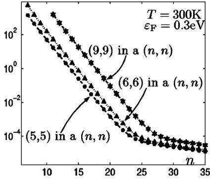
FIG. 8. The transresistance per length  $R_{21}/L$  versus radius ( $r \propto n$ ) for armchair tubes. The different outer and inner armchair tubes are: A (5,5) in a  $(n,n)$  (dots), a (6,6) in a  $(n,n)$  (triangles) and a (9,9) in a  $(n,n)$  (stars). The radius of the outer tube is:  $r = \sqrt{3}a/2\pi n$  for a  $(n,n)$  tube. Here  $T=300$  K and  $\epsilon_F^{(1)} = \epsilon_F^{(2)} = \epsilon_F = 0.3$  eV is used. Note the logarithmic scale.
