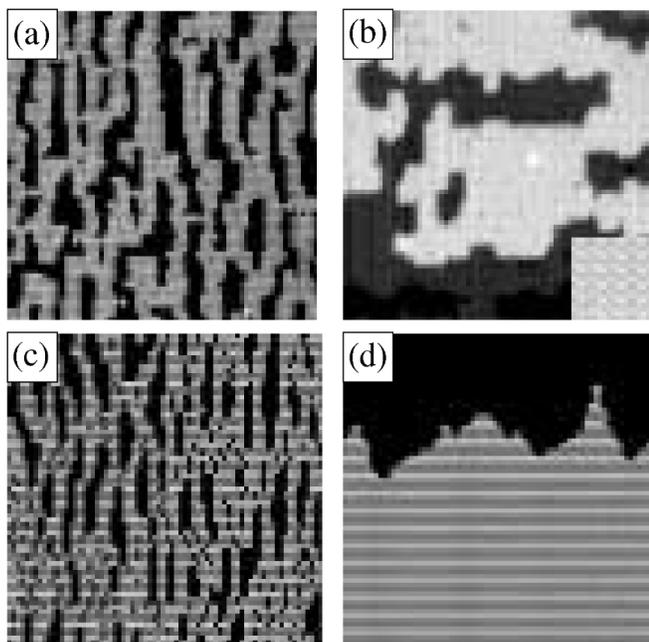
FIG. 2. STM images of Pt(110) at a CO coverage of (a)  $\approx 0.8$  and (b) 1, the latter imaged in a  $10^{-7}$  Torr CO background. The inset shows individual CO molecules in the  $(2 \times 1)$  structure. The images are taken at 300 K as explained in the text. (c),(d) Snapshots from a Monte Carlo simulation of the surface structure at 300 K and at the same two coverages. All parameters are deduced from DFT calculations.
