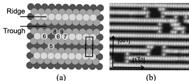
FIG. 1. (a) Model of the missing-row Pt(110)-( $1 \times 2$ ) reconstructed surface. Pt coordination numbers for the perfect surface as well as for various defects are also shown. (b) STM image showing both the clean Pt(110) structure and the first steps in the transformation observed upon CO exposure at RT.
