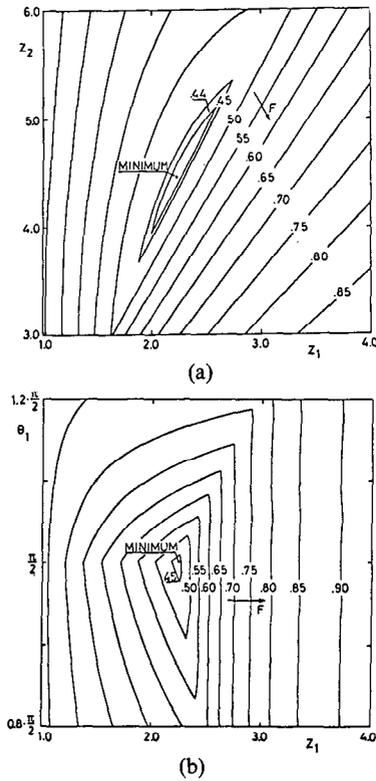
Fig. 2. Two-dimensional ( $n=2$ ) minimax problems arising from optimization of two-section transmission-line 10:1 transformers over 100-percent bandwidth. (a) Singular problem,  $r=2$ . Variation of  $Z_1$  and  $Z_2$ ,  $\theta_1 = \theta_2 = \pi/2$ . (b) Regular problem,  $r=3$ . Variation of  $Z_1$  and  $\theta_1$ ,  $Z_2 = 10/Z_1$ ,  $\theta_2 = \theta_1$ .
