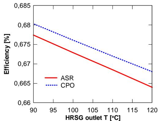
Figure 4. Thermal efficiencies as function of HRSG outlet gas temperature.
