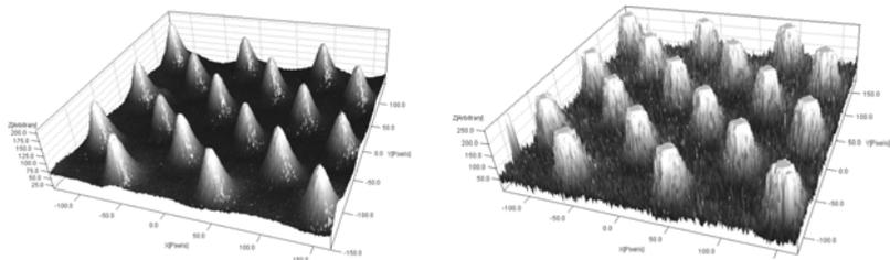
Figure 1: 3D rendering of the calibrated artifact from SEM images with  $HV=5.0$  kV and  $SS=7.0$  nm (left) and  $HV=10$  kV and  $SS=4.0$  nm (right) both at  $M=10000x$ . Qualitatively, the optimum parameters setting results  $HV=10.0$  kV and  $SS=4.0$  nm.
