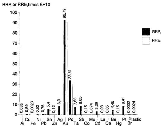
Fig. 2. The resource recovery potential and - efficiency.
