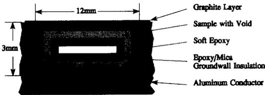
Fig.3 Cylindrical, airfilled void with dielectric/dielectric boundaries. Implemented in the test bar groundwall insulation.
