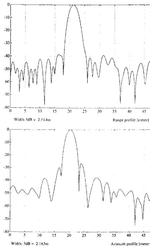
Fig. 4. Point target intensity profiles in dB.
