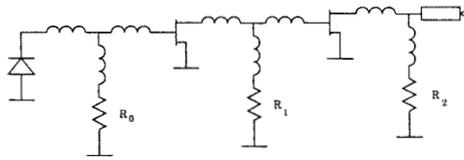
**Figure 1.** Schematic circuit diagram of the front-end amplifier.
