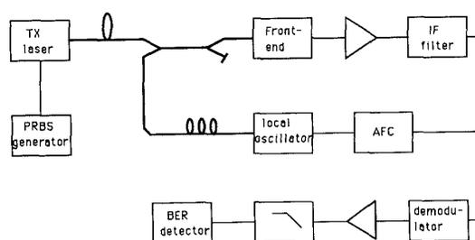
**Figure 5.** Experimental set-up of the 2.5 Gbit/s CPFSK coherent optical system experiment.
