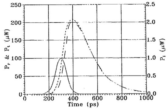
FIG. 2. Power of reflected (short-dashed), transmitted (long-dashed) and input pulses (solid). The input pulse have a FWHM of 100 ps and a peak power of  $1 \mu\text{W}$ .  $\kappa L = 3.0$ ,  $I/I_{th} = 99\%$ .  $P_i$ ,  $P_r$ , and  $P_t$  represent the power of input, reflected, and transmitted pulses, respectively.
