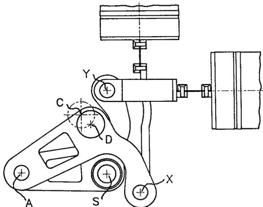
Fig. 3.3. Crank mechanism developed for the heat pump.
