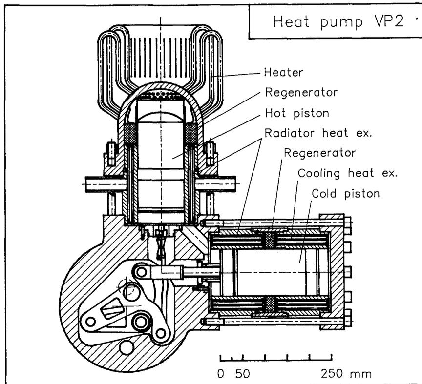
Fig. 4.2. The new 20 kW heat pump VP2.
