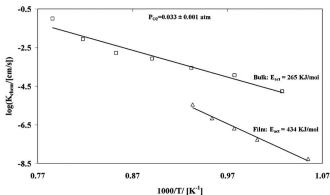
**Figure 10.** Arrhenius-type plot of the chemical exchange coefficient,  $K_{\text{chem}}$ , of LSF64 film and values for a bulk sample from Sogaard et al.<sup>18</sup>
