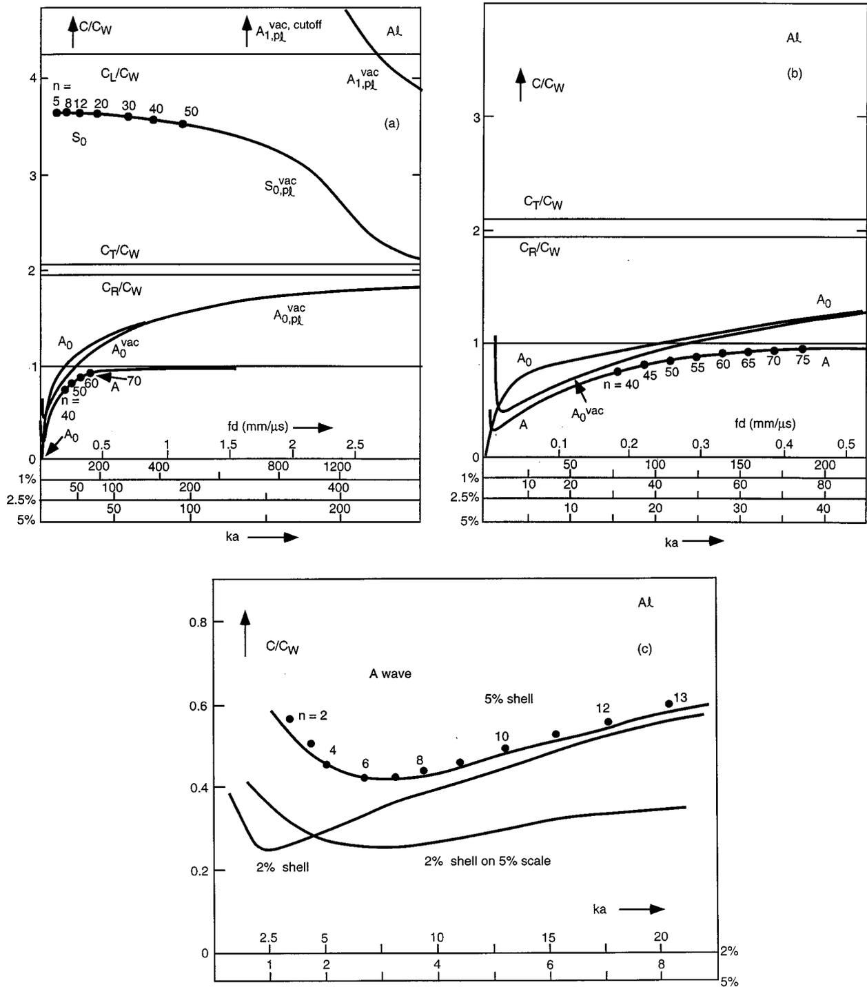
FIG. 4. Comparison of calculated dispersion curves on water-loaded, evacuated spherical aluminum shells with results obtained from calculated resonance frequencies (5% thickness); (a) for  $A$ ,  $A_0$ , and  $S_0$  waves ( $A_1$  wave also indicated); (b) for  $A$  and  $A_0$  waves on an extended scale; (c) for the  $A$  wave, further extended scale and 2% shell curve added.
