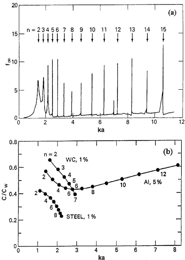
FIG. 2. (a) Resonances in the form function ( $\equiv$ far field backscattering amplitude) of an air-filled aluminum shell in water, of thickness 5%, plotted vs  $ka$ . (b) Dispersion curve of the *A* wave on the aluminum shell, plotted vs  $ka$ . Also shown are portions of the dispersion curves for 1% steel and 1% WC shells. From Ref. 2.
