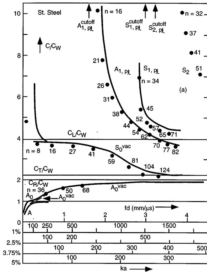
FIG. 5. Comparison of calculated dispersion curves on water-loaded, evacuated spherical stainless steel shells with results obtained from calculated resonance frequencies: (a) for  $A$ ,  $A_0$ ,  $S_0$ ,  $A_1$ , and  $S_1$  waves ( $S_2$  wave also indicated), 5% thickness; (b) for  $A$  and  $A_0$  waves at 2.5% thick shells (1% resonance points added).
