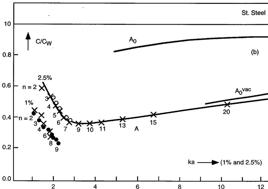
The results for the 2.5% steel shell as shown here demonstrate the low-frequency upturn of the  $A$  wave, as noted earlier for the Al shell; cf., e.g., Fig. 4(c). By comparison with the 5% and 2%  $A$  curves for Al, Fig. 5(b) shows analogous 2.5% and 1%  $A$  curves for steel, and by this analogy, it becomes clear that the Junger wave on a 1% steel shell is the low-frequency upturning extension of the  $A$ -wave dispersion curve of the water-loaded shell.<sup>28</sup>
