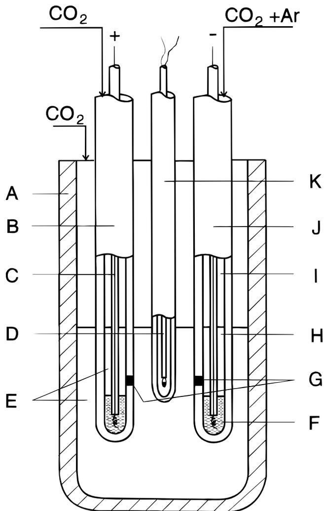
**Figure 1.** Experimental setup for EMF measurements. A, alumina crucible; B, reference electrode chamber; C, alumina tube covered iron wire; D, thermocouple; E, Li/K (43/57) melt; F liquid lead; G, porous alumina diaphragm; H, Li/K melt of various composition; I, alumina tube covered iron wire; J, measuring electrode chamber; and K, alumina tube for thermocouple.
