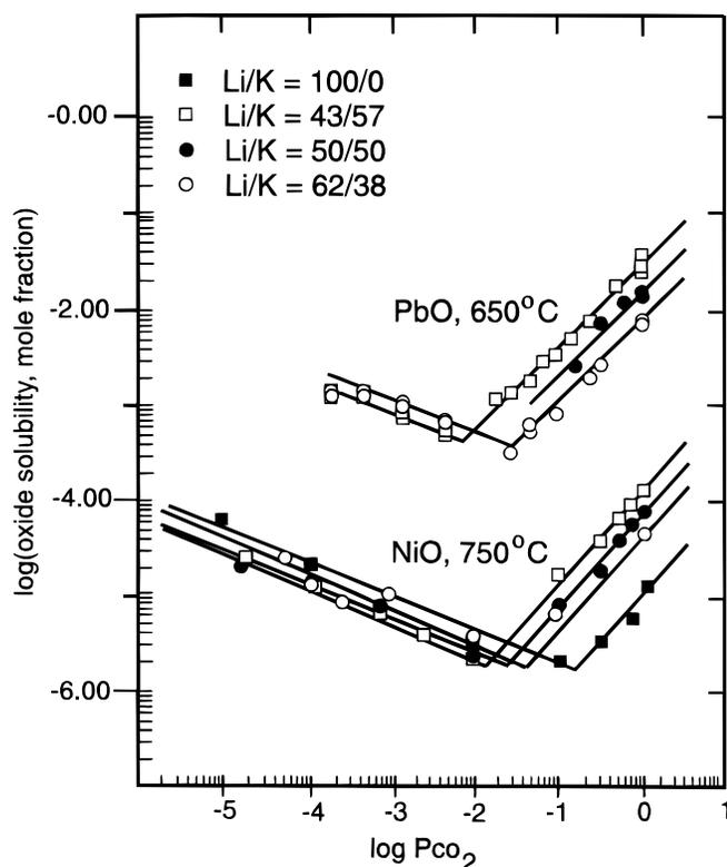
**Figure 4.** Solubility of metal oxides as a function of carbon dioxide partial pressure in Li/K carbonates. PbO data at 650°C from the present work, and NiO data at 750°C from Ota et al.<sup>7</sup> The melt composition is indicated in the figure.
