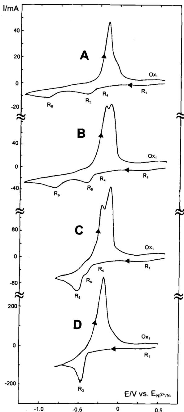
Fig. 3. Cyclic voltammograms at different temperatures of  $K_2NbF_7$  (1.0 m/o) dissolved in eutectic LiCl-KCl melts with KF (1.0 m/o) added. Scan rate: 0.5 V/s. Platinum working electrode (0.047  $cm^2$ ), vitreous carbon counterelectrode, and  $NiCl_2$  (1 m/o)/Ni reference electrode. Temperatures: A, 370°C; B, 450°C; C, 520°C; D, 660°C.
