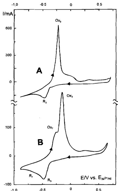
Fig. 9. Cyclic voltammograms at 725°C without and with Na<sub>2</sub>O added of K<sub>2</sub>NbF<sub>7</sub> (1.0 m/o) dissolved in LiCl-KCl-KF melt (F/Nb = 7.9). Scan rate: 5 V/s. Platinum working (0.24 cm<sup>2</sup>), counter- and reference electrodes. Molar ratios O/Nb: A: 0, B: 1.08.
