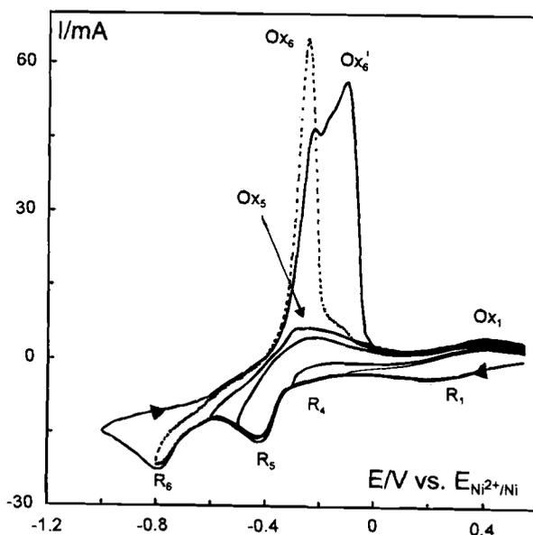
Fig. 4. Cyclic voltammograms at 450°C with different cathodic reverse potentials of  $K_2NbF_7$  (1.0 m/o) dissolved in eutectic LiCl-KCl melts with KF (1.0 m/o) added. Platinum working electrode (0.047  $cm^2$ ), vitreous carbon counterelectrode, and  $NiCl_2$  (1 m/o)/Ni reference electrode. Scan rate: 0.5 V/s.
