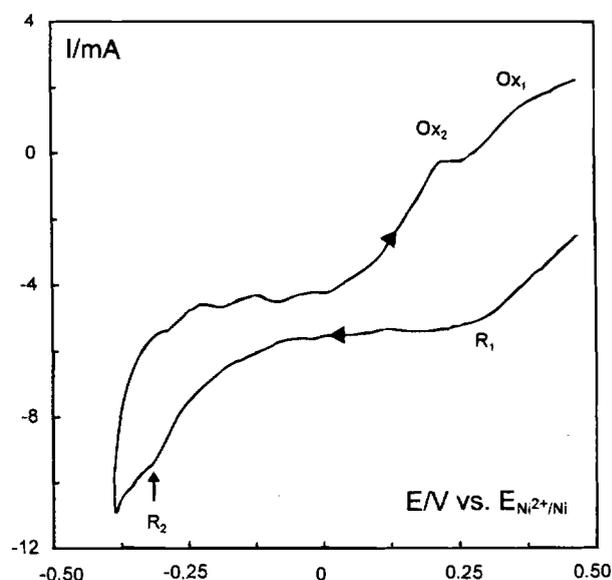
Fig. 2. Cyclic voltammogram at 725°C of K<sub>2</sub>NbF<sub>7</sub> (1.1 m/o) dissolved in eutectic LiCl-KCl melt with KF (1.0 m/o) added. Scan rate: 0.5 V/s. Platinum working (0.024 cm<sup>2</sup>), counter- and reference electrodes.
