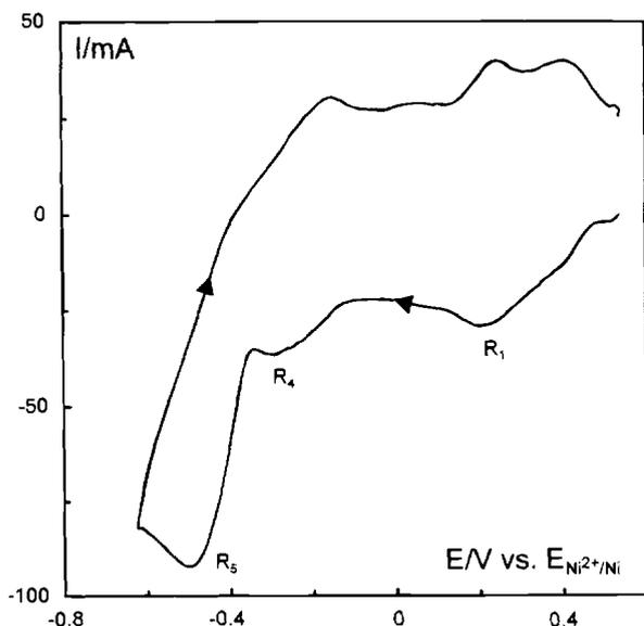
Fig. 5. Cyclic voltammogram at high scan rate of eutectic LiCl-KCl melt at 450°C with  $\text{K}_2\text{NbF}_7$  (1.0 m/o) and KF (1.0 m/o) added. Platinum working electrode, vitreous carbon counterelectrode, and  $\text{NiCl}_2$  (1 m/o)/Ni reference electrode. Scan rate: 20 V/s.
