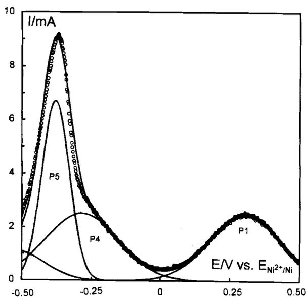
Fig. 8. Square wave voltammogram at 450°C of  $K_2NbF_7$  (1.0 m/o) dissolved in eutectic LiCl-KCl melt with KF (1.0 m/o) added. Scan rate: 0.1 V/s, frequency: 50 Hz, square wave amplitude: 15 mV. Platinum working electrode, vitreous carbon counterelectrode, and  $NiCl_2$  (1 m/o)/Ni reference electrode. Dotted line: measured current. Full lines: simulated waves.
