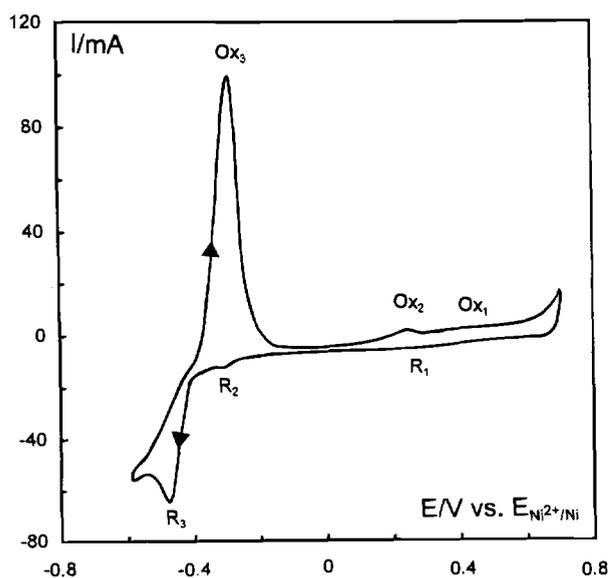
Fig. 1. Cyclic voltammogram at 725°C of K<sub>2</sub>NbF<sub>7</sub> (1.1 m/o) dissolved in eutectic LiCl-KCl melt with KF (1.0 m/o) added. Scan rate: 0.5 V/s. Platinum working (0.024 cm<sup>2</sup>), counter- and reference electrodes.
