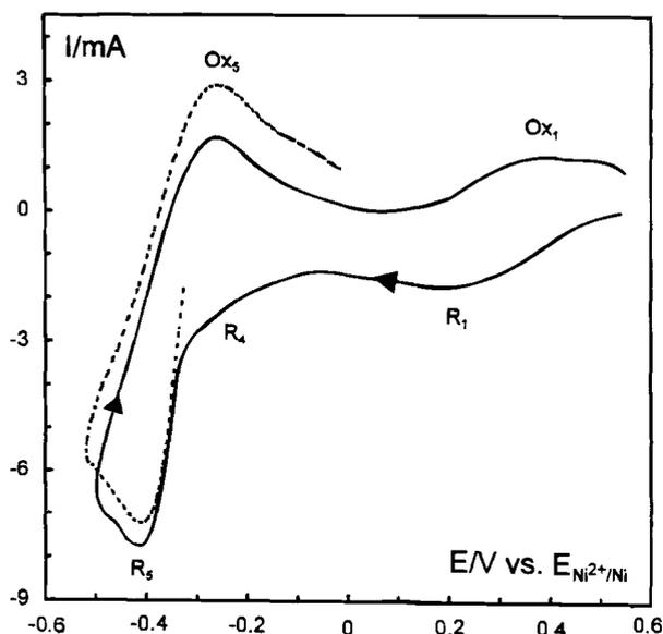
Fig. 7. Cyclic voltammograms (see text) at 450°C of eutectic LiCl-KCl melt with  $K_2NbF_7$  (1.0 m/o) and KF (1.0 m/o) added. Scan rate: 50 mV/s. Platinum working electrode, vitreous carbon counterelectrode, and  $NiCl_2$  (1 m/o)/Ni reference electrode. Full line: normal conditions. Dotted line: initial potential of  $-0.3$  V applied for 10 s before recording.
