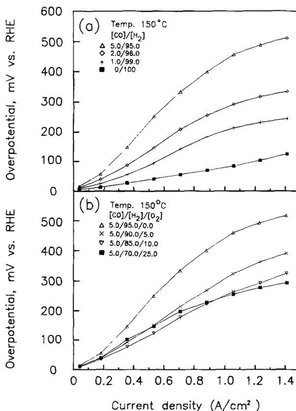
Fig. 2. Polarization curves for hydrogen oxidation in 100 w/o  $\text{H}_3\text{PO}_4$  at 150°C. (a) Hydrogen and hydrogen containing CO; (b) mixture of hydrogen and CO in the presence of  $\text{O}_2$ .
