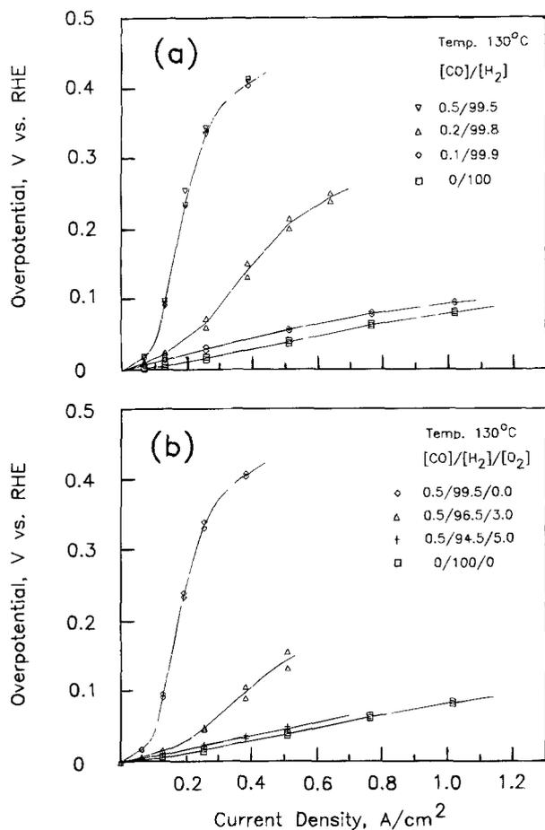
Fig. 3. Polarization curves for hydrogen oxidation in 100 w/o  $\text{H}_3\text{PO}_4$  at 130°C. (a) Hydrogen and hydrogen containing CO; (b) mixture of hydrogen and CO in the presence of  $\text{O}_2$ .
