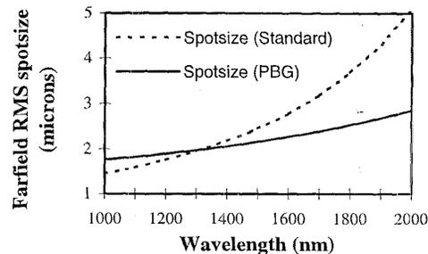
The standard fibre has the same core-cladding refractive-index difference as the PCF at the wavelength  $\lambda = 1.3 \mu\text{m}$ , and a core diameter of  $\Lambda$ . An important observation from this comparison is that the PCF has a much weaker wavelength dependency than the standard fibre.
