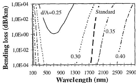
These results indicate that a large operational wavelength range (of interest to optical communications) is available with PCFs, which in addition have the perspective of providing very low scattering losses, because they may be fabricated from undoped silica.
