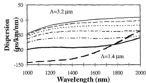
For the fibre parameter range used in Figure 4, it is noteworthy that the effective normalised frequency [2],  $V_{\text{eff}}$ , is in the range from 2.0 to 3.5 (smallest value for smallest pitch). This should be compared to the result of [3], where it is found that a PCF with  $V_{\text{eff}} < 2.5$  could be expected to support only a single mode.
