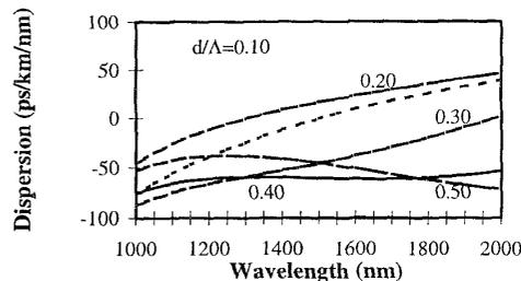
From Figure 3 we first note that for very small air filling fractions, e.g., when the influence of the air holes are strongly limited, the dispersion curve is expectedly very close to the material dispersion of pure silica (zero dispersion wavelength around  $1.3 \mu\text{m}$ ). As the diameter of the air
