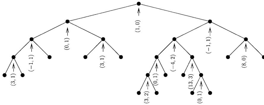
Fig. 3. Free tree for test image c04a200 ( $b = 4000$  b). The cost of coding the data is 493 328 b. The cost of coding the structure of the tree is 25 b. To code the 12 split pixels, which are stored in the internal nodes of the tree, we use  $12 \cdot 11$  b. The code string for the tree structure is 1 111 000 100 111 100 010 100 100.
