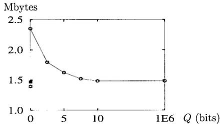
Fig. 5. Comparison between FPAC-B (nonfilled square) and “FPAC-B” using a context selection rule similar to that of the context algorithm [4] with bias  $Q$  (circle). Default pixel ordering (1-norm). Parameters for both coders are  $l = 31$ ,  $N_{St} = 349\,525$ ,  $T_{ca} = 0$ . The pure PMDL context selection [4] corresponds to  $Q = 0$ . Bias  $Q = \infty$  corresponds to a leaf coder. The filled square displays the FPAC-B total with  $l = 24$ ,  $N_{St} = 87\,381$ ,  $T_{ca} = 0$ .
