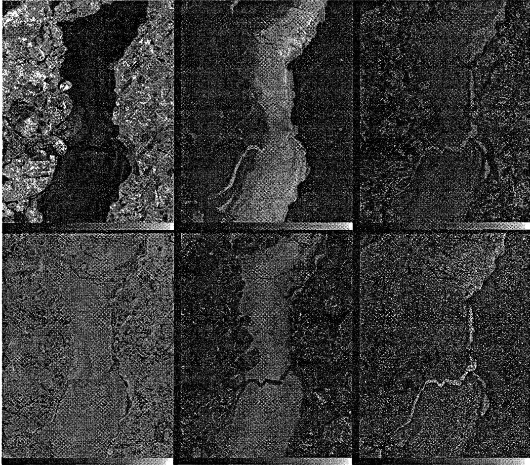
Figure 1. EMISAR polarimetric C-band signature maps of sea ice observed in the Greenland Sea, March 1995. All signatures map are scaled linear within specified ranges (from upper left to right):  $\sigma_{hh}^0$ [-30:-10 dB],  $r_{cp}$ [-5:10 dB],  $r_{xp}$ [-15:0 dB],  $|\rho_{hhvv}|$ [0:1],  $\varphi_{hhvv}$ [-30:90°], and  $\delta_1$  [0:2].
