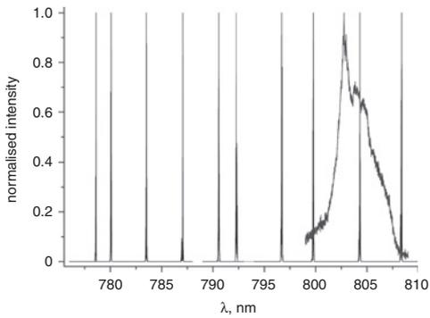
**Fig. 4** Wavelength tuning for pulsed external cavity tapered laser at 20°C
