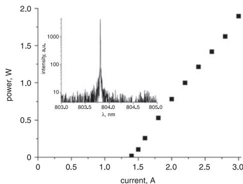
Fig. 2 Light-current characteristics for external cavity tapered laser in CW operation at 20°C
