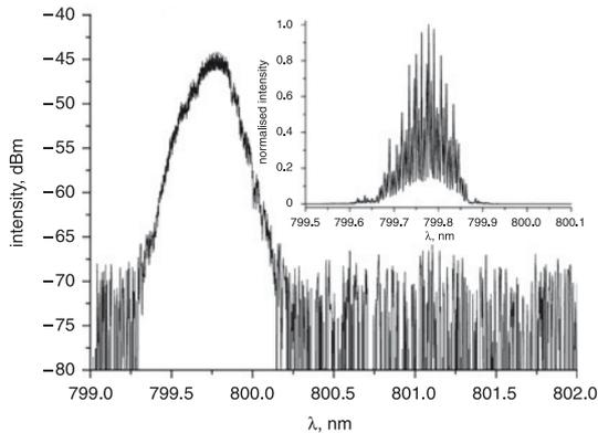
**Fig. 5** Spectrum of external cavity tapered laser in pulsed operation with 20 W peak power at 20°C and with 60 ns pulse width at 500 Hz repetition rate
