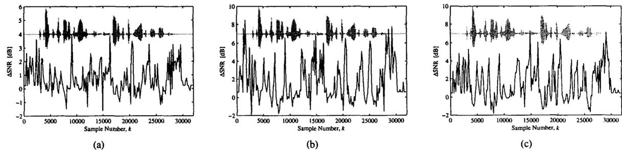
**Figure 7** (a) Difference between segmental SNRs of enhanced speech (MV estimator) obtained by the RRULVD and the SVD, i.e.,  $SNR_{RRULVD}/SNR_{SVD}$ . (b) As (a) but in the colored noise case obtained by the RRULLVD and the QSVD, i.e.,  $SNR_{RRULLVD}/SNR_{QSVD}$ . (c) Difference between segmental SNRs of enhanced speech (MV estimator) obtained by the RRULVD using a sliding and exponential window ( $\beta = 0.99$ ), respectively, i.e.,  $SNR_{sl}/SNR_{exp}$ .
