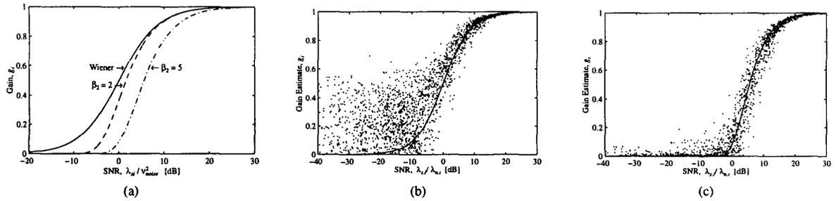
**Figure 1** (a) Wiener and SDC gain functions for different choices of  $\beta_2$ . (b) Estimated Wiener gains  $\{g_i\}_{i=1}^{12}$  of 165 speech frames ( $\mathbf{X} \in \mathbb{R}^{141 \times 20}$ ) obtained from a noisy speech sentence (white noise and SNR=10dB). (c) For the SDC estimator ( $\beta_2 = 5$ ).
