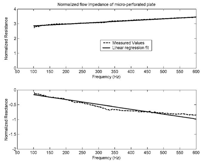
FIG. 3. Real and imaginary part of measured flow impedance of the Acustimet sample, and linear fits. The data are normalized with  $\rho_0 c_0$ .
