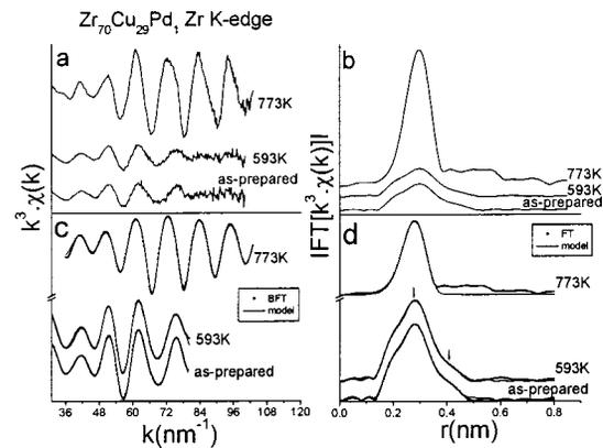
FIG. 3. (a) Experimental  $k^3 \cdot \chi(k)$  for  $Zr_{70}Cu_{29}Pd_1$  alloy in as-prepared stage and after pre-annealing at 593 and 773 K measured above Zr edge, (b) Fourier transforms of (a), (c) Fourier filtered signal (dots) from selected number of shells and simulated EXAFS spectra (line), and (d) Fourier transforms of (c).
