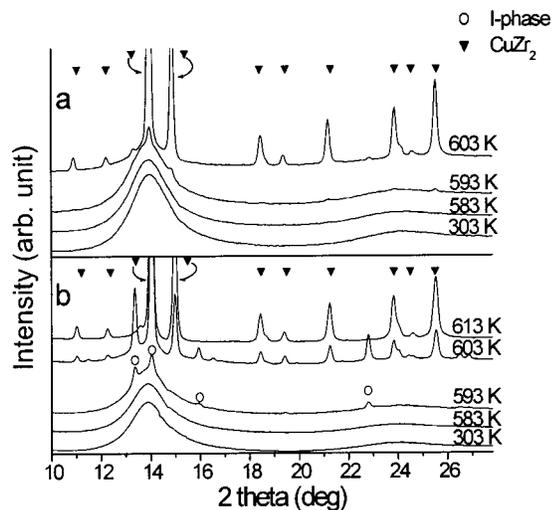
FIG. 1. *In situ* high-temperature XRD patterns of (a)  $Zr_{70}Cu_{30}$  and (b)  $Zr_{70}Cu_{29}Pd_1$  ribbon samples using a wavelength of 0.05904 nm.
