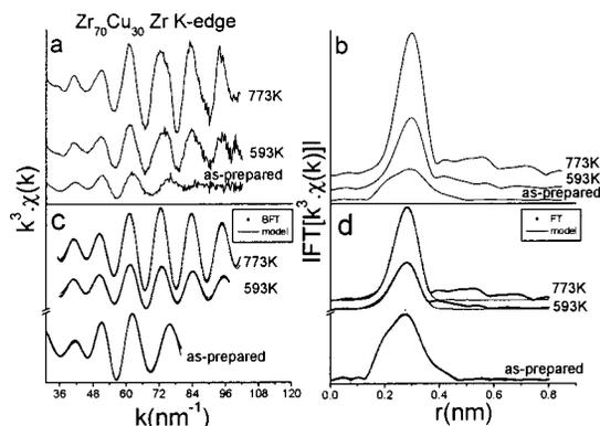
FIG. 4. (a) Experimental  $k^3 \cdot \chi(k)$  for  $Zr_{70}Cu_{30}$  alloy in as-prepared stage and after pre-annealing at 593 and 773 K measured above Zr edge, (b) Fourier transforms of (a), (c) Fourier filtered signal (dots) from selected number of shells and simulated EXAFS spectra (line), and (d) Fourier transforms of (c).
