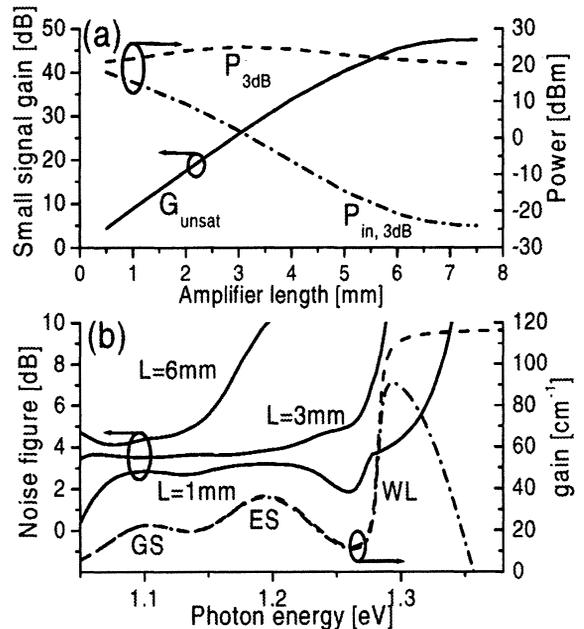
**Fig.1:** (a) Small signal gain and input and output power required to reduce the gain by 3dB. (b) Noise figure for different device lengths and gain spectrum under full inversion (dashed line) and for a current density of  $1.75\text{kA}/\text{cm}^2$  (dash-dotted line).
