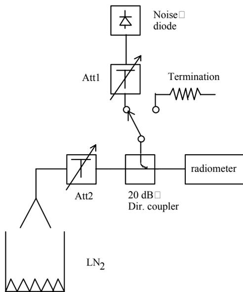
Fig. 3: Slope measurement set-up
