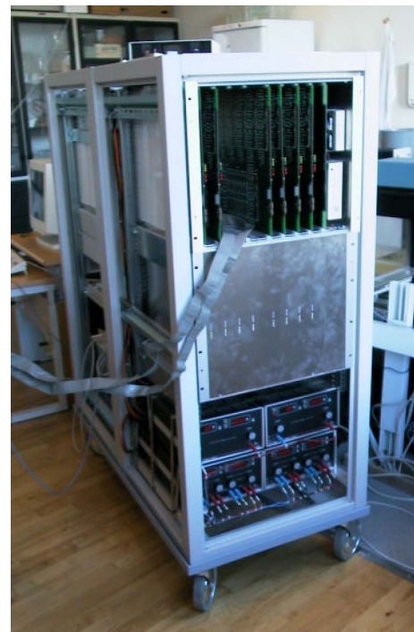
Figure 4: The RASMUS scanner seen from the front with the receivers on the top, transmitters in the middle and the power supplies in the bottom.
