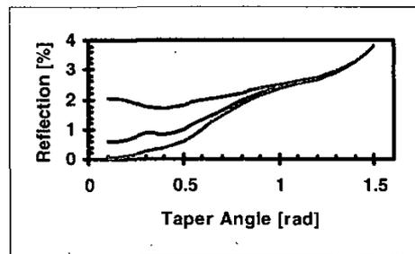
Fig. 2, Reflection versus taper angle for three different circle radii,  $r'$  in Fig. 1, the upper trace  $r'=165 \text{ nm}$  the middle trace  $r'=8 \text{ nm}$  and the lower trace  $r'=25 \text{ nm}$
