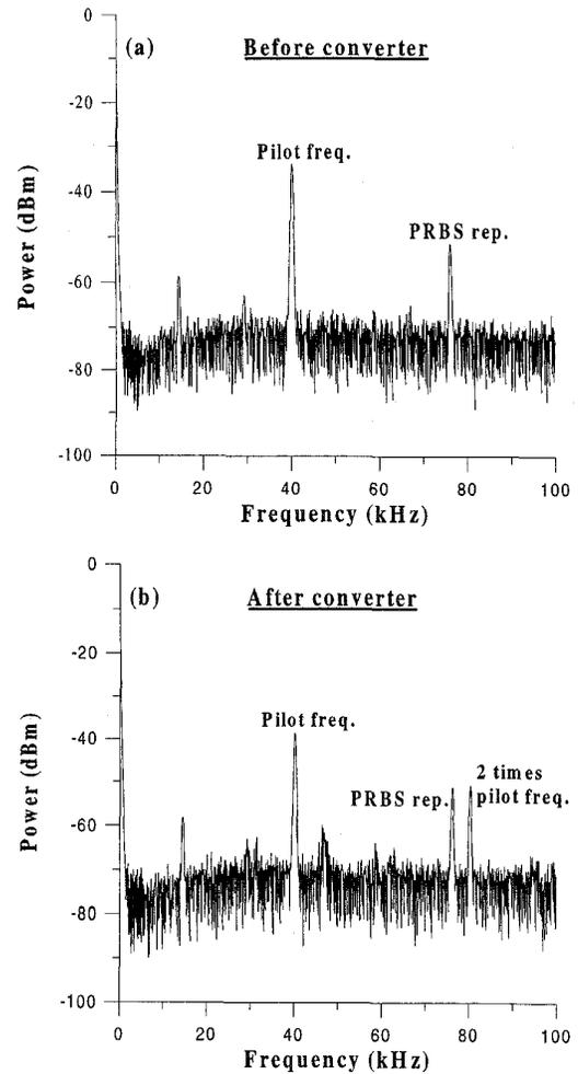
TuE6 Fig. 2. Low-frequency spectrum (a) before and (b) after the IWC. Pilot tone frequency: 40 kHz; electrical bandwidth: 300 kHz.
