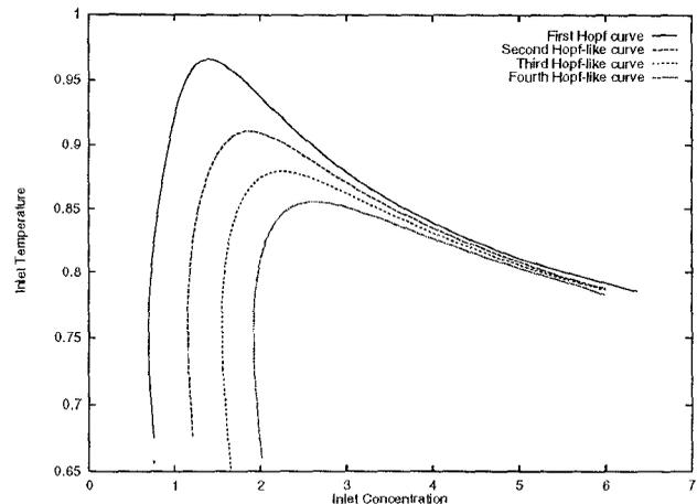
Figure 2: Bifurcation diagram for fixed bed reactor with mass recycle
