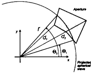
Figure 1: Definition of distances and angles in the aperture plan for evaluating the Rayleigh integral.
