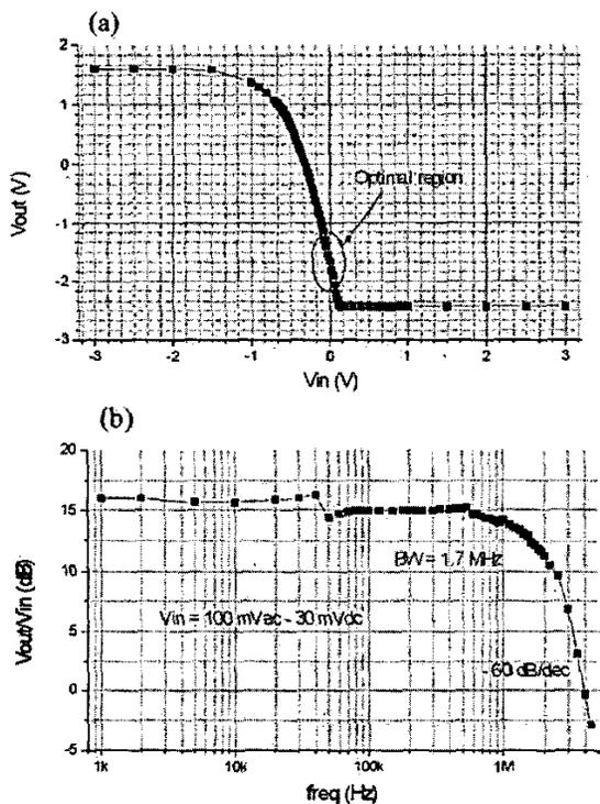
Figure 3: Characterization results of the amplification circuit described in the text. (a) The  $V_{out}$  versus  $V_{in}$  showing the linear region where the circuit has the optimal gain and (b) the frequency response of the circuit showing that the bandwidth is 1.7MHz.
