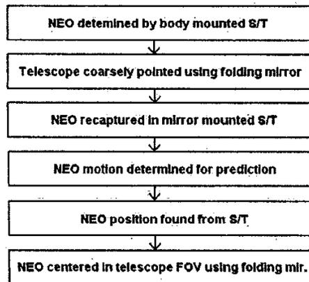
Fig. 5: Flow diagram showing the operational flow from the detection of the NEO to the acquisition of the telescope
