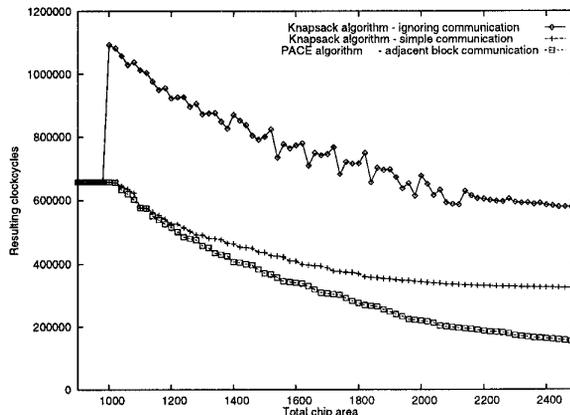
Figure 7: The PACE algorithm compared with Knapsack algorithms which ignore communication or do not account for adjacent hardware block communication optimization (allocation A).
