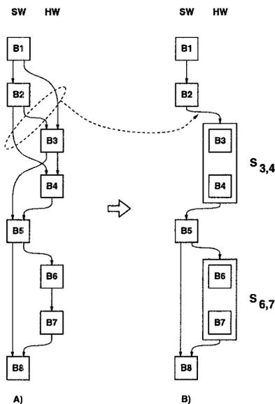
Figure 3: Partitioning model used by PACE: a) Example of actual data-dependencies between hardware and software BSBs, b) How data-dependencies between adjacent hardware BSBs and software BSBs are interpreted in the model.
