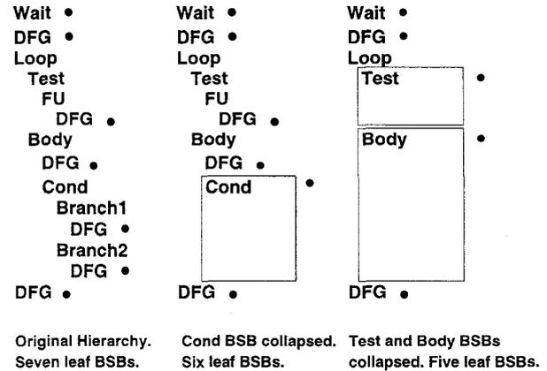
Figure 2: Adjusting BSB granularity by hierarchical collapsing.
